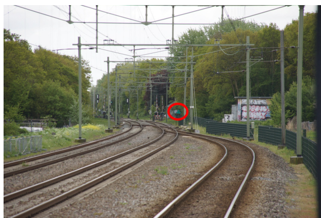
Figure 153: Downstream towards Hlm the speed sign is incorrectly drawn on the OBE. The OBE visualizes a standard 10 speed sign, while it should be a triangle accelerate to 10 speed sign.
