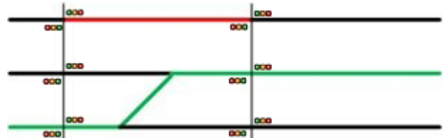
Figure 18: The "demand" switch example on open track. Sometimes the interlocking needs to prohibit a train on the third red track when a train switches to the middle track (green line).
